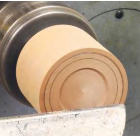
STEP 13. The outer mark is the diameter of the hole in the rosewood and the inner mark is where you are going to hollow the box out to; this should leave a nice, thin wall thickness to the piece
